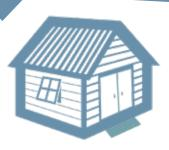
We took our Saltbox shed and gave it some flair. The roofing is upgraded to architectural asphalt shingles with a copper roll ridge cap and the siding is horizontal Eastern White pine clapboard.
